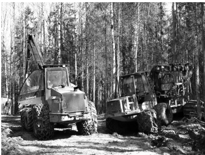
Photo 4. A pair of forwarder and harvester tractor can easily replace logging teams of 20 workers. Photo: Uuve Södör.
