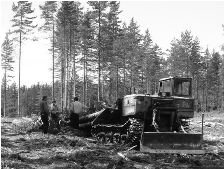
Photo 3. Logging teams are often assigned the motor saw logging technology, and accompanied by the Russian skidding tractor.
